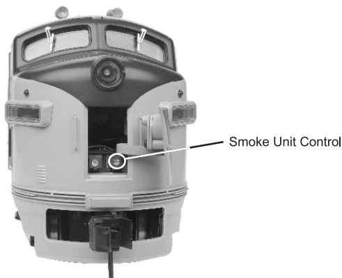
Figure 13: Smoke Unit Switch location
